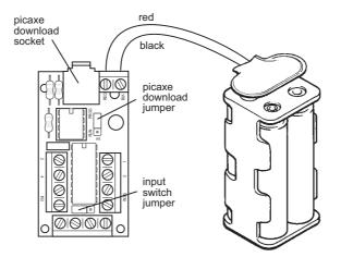
Power should be connected to the board via a battery snap, which can be threaded through the two large holes to create a stronger connection point. The PICAXE-08M2 microcontroller will function at battery voltages between 3 and 5V (do not use a 9V PP3 battery). Most users will use 3xAA alkaline cells (4.5V) or 4xAA rechargeable cells (4.8V).
