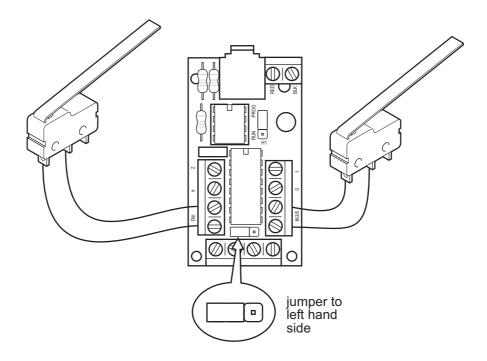
If the jumper link is moved to the right hand position two inputs are then available, C.3 and C.5. However as pin C.5 on the 08M2 chip is also shared as the serial programming pin you must ensure that the switch is not pressed during programming, or during powerup of the circuit. You must also include a 'disconnect' command at the start of your BASIC program - please see the main PICAXE manual for more details about this configuration and use of the disconnect command.
