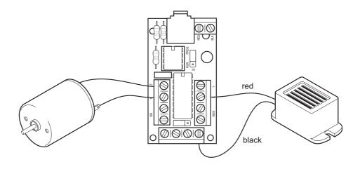
The outputs can be used individually to driver electronic devices such as buzzers and signal lamps. To connect outputs in this way the red wire is connected to the terminal block at the side of the board and the black wire is connected to 0V (G) at the bottom of the board.
