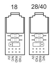
The adapter supports the standard download circuit (10k and 22k resistor) and has a 2 way jumper to allow ease of layout of 18 and 28/40 pin PICAXE circuits on the breadboard.
